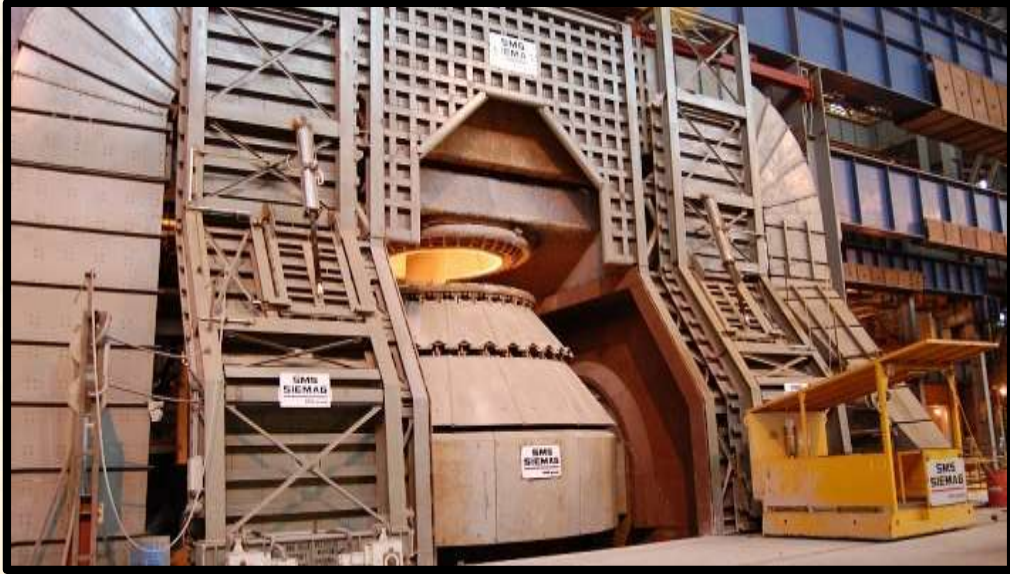
LD Converters for Vishakhapatnam Steel Plant 6.3 MTPA Expansion Project of Rashtriya Ispat Nigan Ltd.
